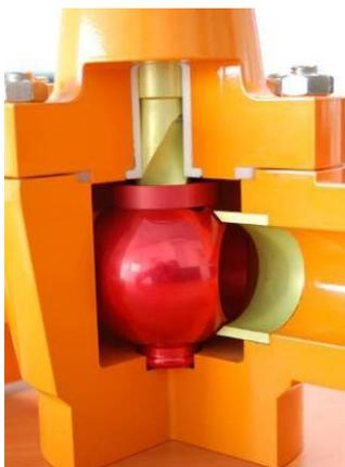
As the stem lowers, the special designed helix shaped trunnion causes the ball to start its rotation towards the closed position.
