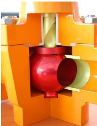
Valve is in full open position and the ball is not in contact with the seat. The stem is at its upper position and the ball is positioned for optimal flow.
